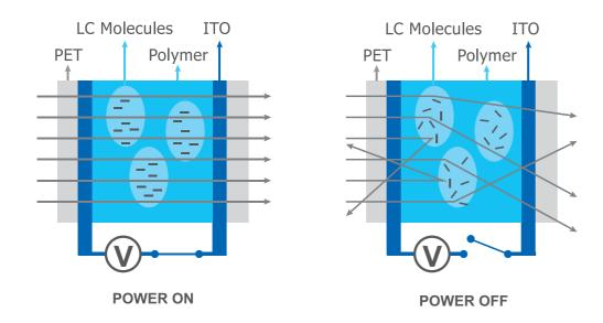
**POWER ON:** LC Molecules are arranged in a regular manner, allowing Light to pass uninterrupted.
